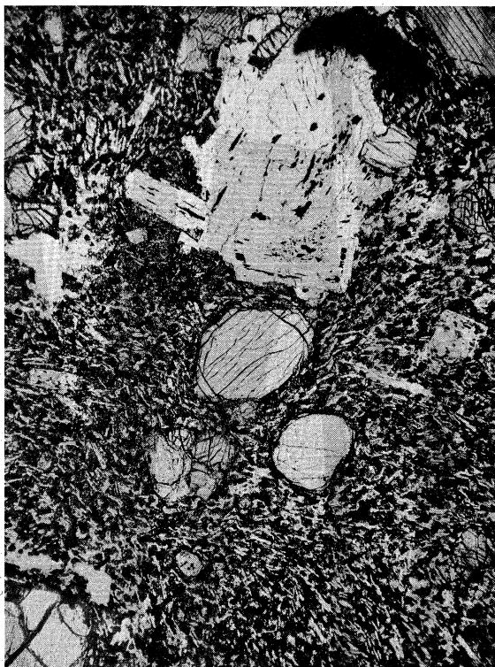
Figure 1: Phenocryst of olivine (centre) in a fine-grained groundmass; olivine basalt from Ookala, Mauna Kea, Hawaii (magnified 28 X).
